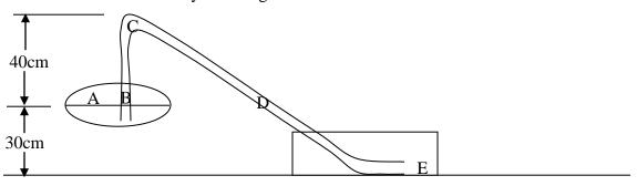
(a) Draw a set of quantitatively accurate energy density bar graphs for point A, at the surface of the gas in the tank (30cm from the ground), and point E, just after the fluid exits the siphon tube. Use them to approximate the rate at which gasoline flows into Greg's tank. Ignore dissipative losses.
