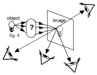
If something is placed in front of the object that scatters the light, such as a frosted glass, your eye will detect the light, but it will not see an image. The light from one point on the object
