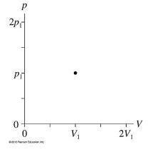
4. A gas starts with pressure  $p_I$  and volume  $V_I$ . Show on the figure the process in which the gas undergoes an isothermal process during which the volume is halved, then an isochoric process during which the pressure is halved, followed by an isobaric process during which the volume is doubled. Label each of the three processes.
