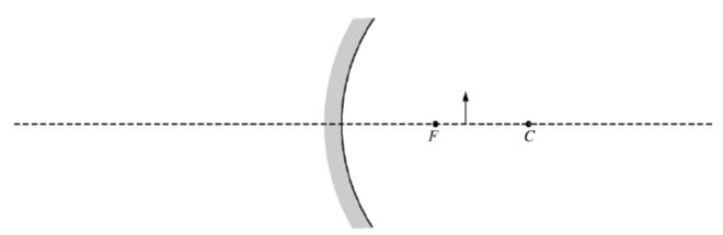
The figure above shows a converging mirror, its focal point F, its center of curvature C, and an object represented by the solid arrow.
