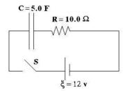
76. For the RC circuit shown, the resistance is  $R = 10.0 \Omega$ , the capacitance is C = 5.0 F and the battery has voltage  $\xi$ = 12 volts. The capacitor is initially uncharged when the switch S is closed at time t = 0. At some time later, the current in the circuit is 0.50 A. What is the magnitude of the voltage across the capacitor at that moment? (A) 5 volts (B) 6 volts (C) 7 volts (D) 12 volts
