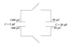
71. For the configuration of capacitors shown, both switches are closed simultaneously. After equilibrium is established, what is the charge on the top plate of the 5  $\mu$ F capacitor?
