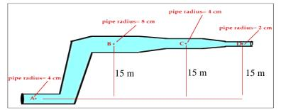
27. The pressure at A is 9.5 atm and the water velocity is 10 m/s. What is the water velocity at point C?
