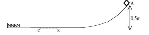
6. A 2 kg block is dropped from rest at point A. The spring constant is k = 500 N/m. Assume no friction. What is the maximum compression of the spring?
