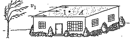
FIG. 14.10. Air blowing across a roof causes the pressure to be reduced. If the wind blows fast enough, the internal air pressure can blow the roof off.
