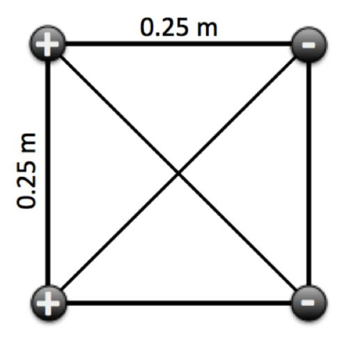
Four charges are arranged in a square with sides of length 0.25m. All four charges have a magnitude of 6.0µC and their type of charge is labeled on the diagram above. What is the magnitude of the electric field at the center of the square?
