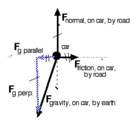
2. Here's a very different looking situation, but the analysis is very similar. In fact, turning the previous force diagram 180 degrees results in the force diagram shown. Realizing that all force diagrams have many similarities can be a relief. You don't need to memorize a bunch of different approaches to be able to draw a wide variety of force diagrams.
