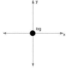
**Step 4.** Proceed around the system boundary line and identify all points at which there is contact between the system (log) and its surroundings. Construct qualitative vectors (indicate directions and **relative** magnitudes) to represent these forces.
