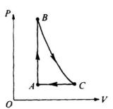
14. Gas in a chamber passes through the cycle ABCA as shown in the diagram above. In the process AB, 12 joules of heat is added to the gas. In the process BC, no heat is exchanged with the gas. For the complete cycle ABCA, the work done by the gas is 8 joules. How much heat is added to or removed from the gas during process CA? (A) 20 J is removed. (B) 4 J is removed. (C) 4 J is added. (D) 20 J is added.
