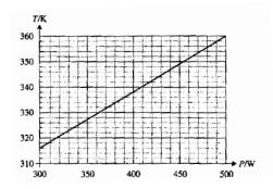
6. The above graph shows the variation with incident solar power P of the temperature of a solar panel used to heat water when thermal energy is extracted from the water at a rate of 320 W. The area of the panel is 2.0 m<sup>2</sup> and the intensity of the solar radiation incident on the panel is 400 W / m<sup>2</sup>. Calculate:
