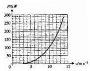
7. The above graph shows the power curve of a wind turbine as a function of the wind speed. If the wind speed is 10 m/s, calculate the energy produced in the course of one year assuming that the wind blows at this speed for 1000 hours in the year.
