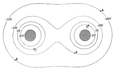
1974B5. The diagram shows some of the equipotentials in a plane perpendicular to two parallel charged metal cylinders. The potential of each line is labeled.
